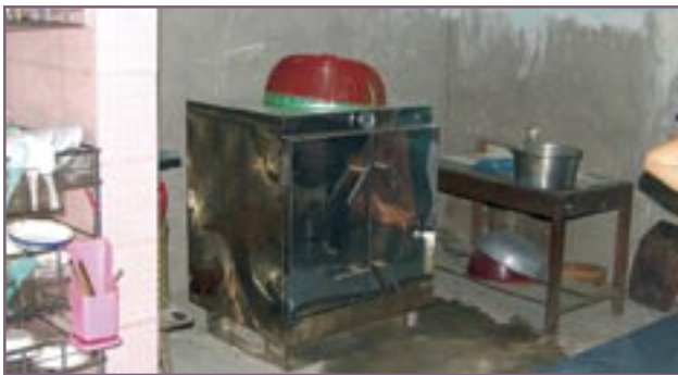
A new large oven is cleaner, more efficient, and safer because of the fire wall behind it.
